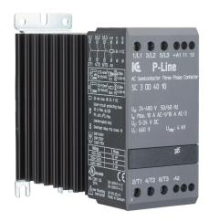
Eltwin SC3 series solid state contactor, 10A, (3) N.O. SCR switched power poles, 24-480 VAC (50/60Hz) operating voltage, 5-24 VDC coil voltage.
