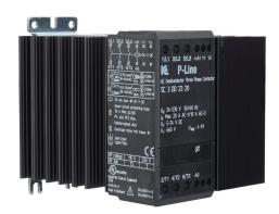
Eltwin SC3 series solid state contactor, 20A, (3) N.O. SCR switched power poles, 12-230 VAC (50/60Hz) operating voltage, 5-24 VDC coil voltage.
