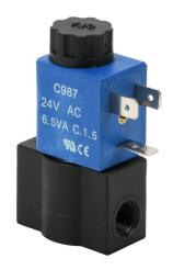
CFA solenoid valve, 2-port (2-way), 2-position, N.C., nylon body, Viton seal(s), 1/8in female NPT inlet(s), 1/8in female NPT outlet(s), Cv=0.28, 0 psi minimum operating pressure, 24 VAC operating voltage, 11mm DIN style wiring plug.
