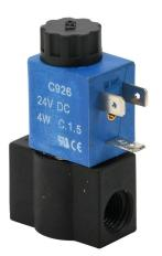
CFA solenoid valve, 2-port (2-way), 2-position, N.C., nylon body, Viton seal(s), 1/4in female NPT inlet(s), 1/4in female NPT outlet(s), Cv=0.14, 0 psi minimum operating pressure, 24 VDC operating voltage, 11mm DIN style wiring plug.
