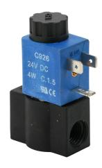
CFA solenoid valve, 2-port (2-way), 2-position, N.C., nylon body, Viton seal(s), 1/4in female NPT inlet(s), 1/4in female NPT outlet(s), Cv=0.14, 0 psi minimum operating pressure, 24 VDC operating voltage, 11mm DIN style wiring plug.
