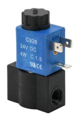
CFA solenoid valve, 2-port (2-way), 2-position, N.C., nylon body, Viton seal(s), 1/8in female NPT inlet(s), 1/8in female NPT outlet(s), Cv=0.28, 0 psi minimum operating pressure, 24 VDC operating voltage, 11mm DIN style wiring plug.
