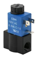
CFA solenoid valve, 2-port (2-way), 2-position, N.C., nylon body, Viton seal(s), 1/4in female NPT inlet(s), 1/4in female NPT outlet(s), Cv=0.28, 0 psi minimum operating pressure, 120 VAC operating voltage, 11mm DIN style wiring plug.
