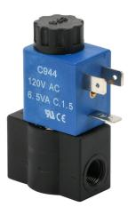
CFA solenoid valve, 2-port (2-way), 2-position, N.C., nylon body, Viton seal(s), 1/8in female NPT inlet(s), 1/8in female NPT outlet(s), Cv=0.28, 0 psi minimum operating pressure, 120 VAC operating voltage, 11mm DIN style wiring plug.
