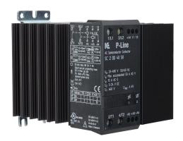
Eltwin SC2 series solid state contactor, 50A, (2) N.O. SCR switched power poles, 24-480 VAC (50/60Hz) operating voltage, 5-24 VDC coil voltage.
