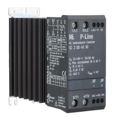
Eltwin SC2 series solid state contactor, 30A, (2) N.O. SCR switched power poles, 24-480 VAC (50/60Hz) operating voltage, 5-24 VDC coil voltage.
