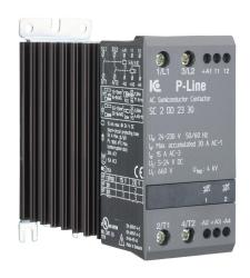
Eltwin SC2 series solid state contactor, 30A, (2) N.O. SCR switched power poles, 12-230 VAC (50/60Hz) operating voltage, 5-24 VDC coil voltage.
