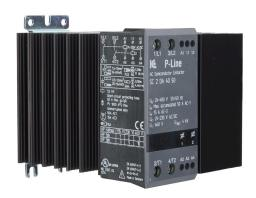
Eltwin SC2 series solid state contactor, 50A, (2) N.O. SCR switched power poles, 24-480 VAC (50/60Hz) operating voltage, 24-230 VAC/VDC coil voltage.
