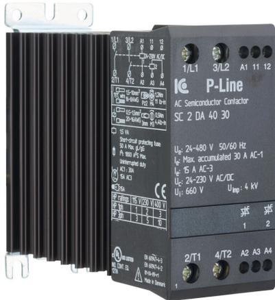
Eltwin SC2 series solid state contactor, 30A, (2) N.O. SCR switched power poles, 24-480 VAC (50/60Hz) operating voltage, 24-230 VAC/VDC coil voltage.
