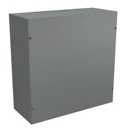
Wiegmann enclosure, NEMA 1, 24 x 24 x 10in (HxWxD), wall mount, with knockouts, carbon steel, ANSI 61 gray, powder coat finish, screw cover.
