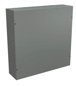
Wiegmann enclosure, NEMA 1, 24 x 24 x 6in (HxWxD), wall mount, with knockouts, carbon steel, ANSI 61 gray, powder coat finish, screw cover.
