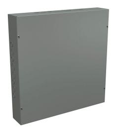
Wiegmann enclosure, NEMA 1, 24 x 24 x 4in (HxWxD), wall mount, with knockouts, carbon steel, ANSI 61 gray, powder coat finish, screw cover.
