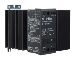
Eltwin SC1 series solid state contactor, 50A, (1) N.O. SCR switched power poles, 24-600 VAC (50/60Hz) operating voltage, 5-24 VDC coil voltage.
