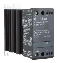
Eltwin SC1 series solid state contactor, 30A, (1) N.O. SCR switched power poles, 24-600 VAC (50/60Hz) operating voltage, 5-24 VDC coil voltage.
