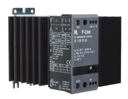
Eltwin SC1 series solid state contactor, 50A, (1) N.O. SCR switched power poles, 12-230 VAC (50/60Hz) operating voltage, 5-24 VDC coil voltage.
