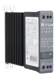
Eltwin SC1 series solid state contactor, 15A, (1) N.O. SCR switched power poles, 12-230 VAC (50/60Hz) operating voltage, 5-24 VDC coil voltage.
