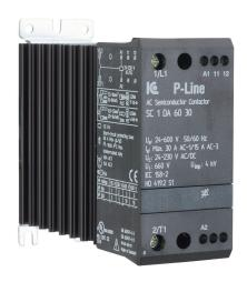
Eltwin SC1 series solid state contactor, 30A, (1) N.O. SCR switched power poles, 24-600 VAC (50/60Hz) operating voltage, 24-230 VAC/VDC coil voltage.
