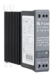
Eltwin SC1 series solid state contactor, 15A, (1) N.O. SCR switched power poles, 24-480 VAC (50/60Hz) operating voltage, 24-230 VAC/VDC coil voltage.
