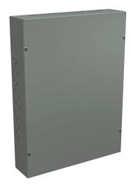
Wiegmann enclosure, NEMA 1, 24 x 18 x 4in (HxWxD), wall mount, with knockouts, carbon steel, ANSI 61 gray, powder coat finish, screw cover.
