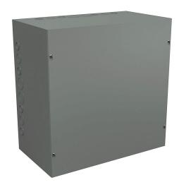
Wiegmann enclosure, NEMA 1, 18 x 18 x 10in (HxWxD), wall mount, with knockouts, carbon steel, ANSI 61 gray, powder coat finish, screw cover.
