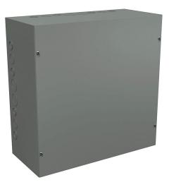
Wiegmann enclosure, NEMA 1, 18 x 18 x 8in (HxWxD), wall mount, with knockouts, carbon steel, ANSI 61 gray, powder coat finish, screw cover.
