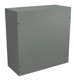
Wiegmann enclosure, NEMA 1, 18 x 18 x 8in (HxWxD), wall mount, carbon steel, ANSI 61 gray, powder coat finish, screw cover.
