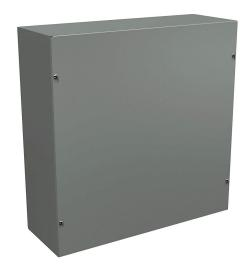
Wiegmann enclosure, NEMA 1, 18 x 18 x 6in (HxWxD), wall mount, carbon steel, ANSI 61 gray, powder coat finish, screw cover
