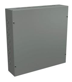
Wiegmann enclosure, NEMA 1, 18 x 18 x 4in (HxWxD), wall mount, with knockouts, carbon steel, ANSI 61 gray, powder coat finish, screw cover.
