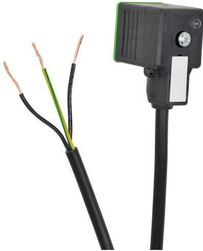
Murrelektronik solenoid valve cable, 18mm DIN 43650 Form A molded connector to 3-wire pigtail, 24 VAC/VDC, 18 AWG, PVC jacket, 16.4ft/5m cable length, surge protection, LED indication.
