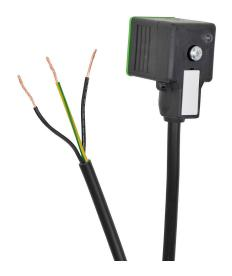
Murrelektronik solenoid valve cable, 18mm DIN 43650 Form A molded connector to 3-wire pigtail, 24 VAC/VDC, 18 AWG, PVC jacket, 16.4ft/5m cable length, surge protection, LED indication.
