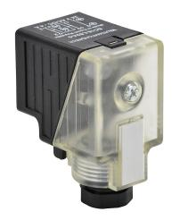
Murrelektronik field wireable solenoid valve connector, 18mm DIN 43650 Form A molded connector, 24 VAC/VDC, 16-12 AWG, accepts cable diameter size 0.24-0.32in, surge protection, LED indication.
