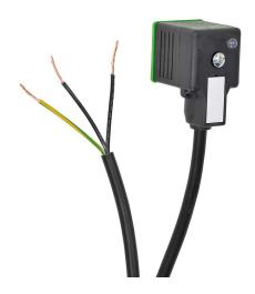
Murrelektronik solenoid valve cable, 18mm DIN 43650 Form A molded connector to 3-wire pigtail, 110 VAC/VDC, 18 AWG, PVC jacket, 16.4ft/5m cable length, surge protection, LED indication.
