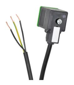
Murrelektronik solenoid valve cable, 18mm DIN 43650 Form A molded connector to 3-wire pigtail, 110 VAC/VDC, 18 AWG, PVC jacket, 9.8ft/3m cable length, surge protection, LED indication.
