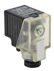
Murrelektronik field wireable solenoid valve connector, 18mm DIN 43650 Form A molded connector, 110 VAC/VDC, 16-12 AWG, accepts cable diameter size 0.24-0.32in, surge protection, LED indication.
