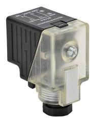
Murrelektronik field wireable solenoid valve connector, 18mm DIN 43650 Form A molded connector, 230 VAC/VDC, 16-12 AWG, accepts cable diameter size 0.24-0.32in.
