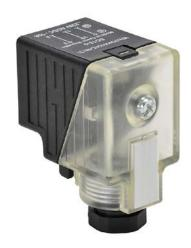
Murrelektronik field wireable solenoid valve connector, 18mm DIN 43650 Form A molded connector, 230 VAC/VDC, 16-12 AWG, accepts cable diameter size 0.24-0.32in.
