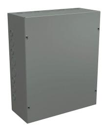
Wiegmann enclosure, NEMA 1, 18 x 15 x 6in (HxWxD), wall mount, with knockouts, carbon steel, ANSI 61 gray, powder coat finish, screw cover.
