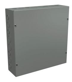
Wiegmann enclosure, NEMA 1, 15 x 15 x 4in (HxWxD), wall mount, with knockouts, carbon steel, ANSI 61 gray, powder coat finish, screw cover.
