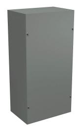
Wiegmann enclosure, NEMA 1, 24 x 12 x 8in (HxWxD), wall mount, carbon steel, ANSI 61 gray, powder coat finish, screw cover.
