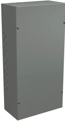
Wiegmann enclosure, NEMA 1, 24 x 12 x 6in (HxWxD), wall mount, with knockouts, carbon steel, ANSI 61 gray, powder coat finish, screw cover.
