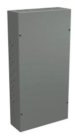
Wiegmann enclosure, NEMA 1, 24 x 12 x 4in (HxWxD), wall mount, with knockouts, carbon steel, ANSI 61 gray, powder coat finish, screw cover.
