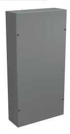
Wiegmann enclosure, NEMA 1, 24 x 12 x 4in (HxWxD), wall mount, carbon steel, ANSI 61 gray, powder coat finish, screw cover.
