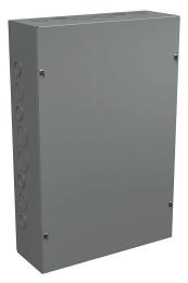
Wiegmann enclosure, NEMA 1, 18 x 12 x 4in (HxWxD), wall mount, with knockouts, carbon steel, ANSI 61 gray, powder coat finish, screw cover.
