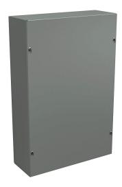
Wiegmann enclosure, NEMA 1, 18 x 12 x 4in (HxWxD), wall mount, carbon steel, ANSI 61 gray, powder coat finish, screw cover.
