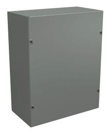
Wiegmann enclosure, NEMA 1, 15 x 12 x 6in (HxWxD), wall mount, carbon steel, ANSI 61 gray, powder coat finish, screw cover.
