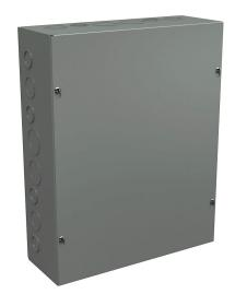
Wiegmann enclosure, NEMA 1, 15 x 12 x 4in (HxWxD), wall mount, with knockouts, carbon steel, ANSI 61 gray, powder coat finish, screw cover.
