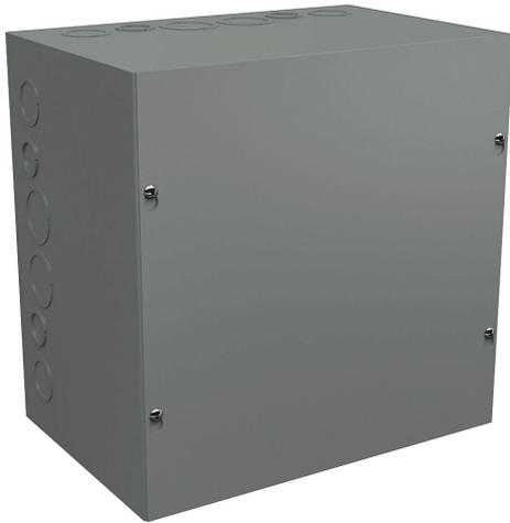
Wiegmann enclosure, NEMA 1, 12 x 12 x 8in (HxWxD), wall mount, with knockouts, carbon steel, ANSI 61 gray, powder coat finish, screw cover.
