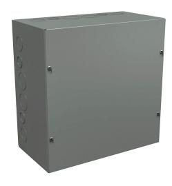
Wiegmann enclosure, NEMA 1, 12 x 12 x 6in (HxWxD), wall mount, with knockouts, carbon steel, ANSI 61 gray, powder coat finish, screw cover.
