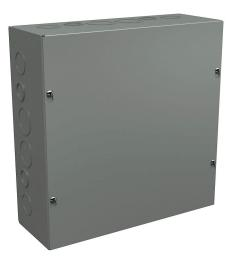
Wiegmann enclosure, NEMA 1, 12 x 12 x 4in (HxWxD), wall mount, with knockouts, carbon steel, ANSI 61 gray, powder coat finish, screw cover.
