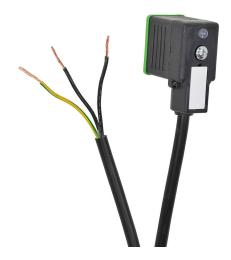
Murrelektronik solenoid valve cable, 11mm DIN style molded connector to 3-wire pigtail, 24 VAC/VDC, 18 AWG, PVC jacket, 16.4ft/5m cable length, surge protection, LED indication.
