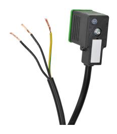
Murrelektronik solenoid valve cable, 11mm reverse DIN style molded connector to 3-wire pigtail, 24 VAC/VDC, 18 AWG, PVC jacket, 16.4ft/5m cable length, surge protection, LED indication.
