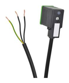
Murrelektronik solenoid valve cable, 11mm DIN style molded connector to 3-wire pigtail, 24 VAC/VDC, 18 AWG, PVC jacket, 9.8ft/3m cable length, surge protection, LED indication.
