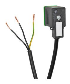
Murrelektronik solenoid valve cable, 11mm reverse DIN style molded connector to 3-wire pigtail, 24 VAC/VDC, 18 AWG, PVC jacket, 9.8ft/3m cable length, surge protection, LED indication.
